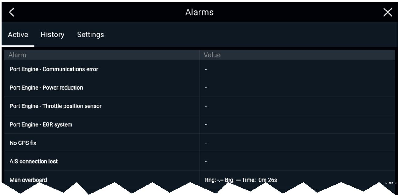
The screenshot shows the 'Alarms' interface with the 'Active' tab selected. It displays a table of active alarms with columns for 'Alarm' and 'Value'. The alarms listed are: Port Engine - Communications error, Port Engine - Power reduction, Port Engine - Throttle position sensor, Port Engine - EGR system, No GPS fix, AIS connection lost, and Man overboard. The 'Man overboard' alarm has a value of 'Rng: -. Brg: — Time: 0m 26s'. A 'Clear history' button is visible in the bottom right corner.
